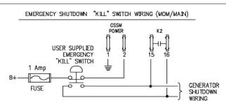
The K1 relay provides a continuous run signal for generators requiring a maintained start signal. The K2 relay provides a momentary stop signal until the generator AC Hz has dropped to zero. For GSCM-mini operational sequence details see page 7, option 2.
