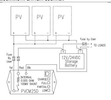
The PVCM25D has an internal shunt for the solar charge current which will handle the maximum of 25 AMPs. The T568A or T568B network patch cable connects the PVCM25D to the PVDM display module. The battery powering the PVCM25D also powers the display module.
