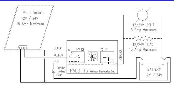
The PVLC-15 charges the battery from the solar PV panel during the day. At dusk the PVLC-15 senses the low PV panel voltage and turns on the light for the selected time period. The light will automatically turn off at dawn. In the Sign option,(switch settings 7,8,& 9) the PVLC-15 also turns on the light two hours before dawn.
