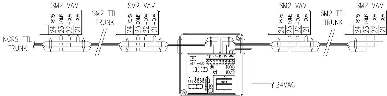
The AETI-485/TTL2 is configured as a SM2 TTL repeater. It can be used to extend an existing communications trunk or split a trunk to eliminate communication problems caused by wire resistance and or capacitance due to long trunk runs. If the RS-485 port is not used, no termination resistor is needed across the AETI's RS-485 terminals (8, 9) because the AETI-485 has a 510 ohm internal impedance resistor on board.
