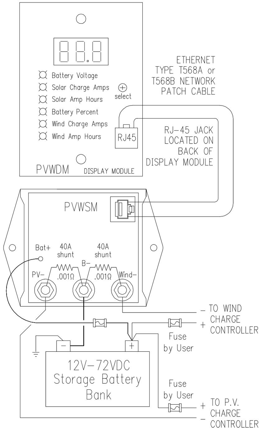
The PVWSM monitors the battery voltage and adjusts the switching power supply to maintain a 12V DC output to power the display module. The PVWSM also contains the 40 amp current shunts to measure the Photo Voltaic charge current and wind charge current in the negative leg. It looks at the voltage drop across the shunts and scales it to a 0 to 2V DC signal. The 12VDC power and shunt signals are fed to the PVWDM through the RJ-45 Jack and network patch cable.
