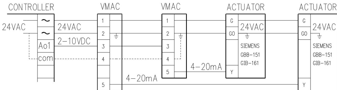
The VMAC inputs may be connected in parallel to share the same DDC 2-10V DC signal and provide individual 4-20mA signals for multiple actuators that share the same power supply. If the total resistance of the actuators is less than 600 ohms, their current inputs may be connected in series if the actuators are powered by separate transformers. Field calibrations may be required due to load resistance variations (see Field Calibration Adjustments above).
