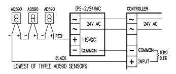
The AD590 sensor when connected in series will perform a lowest temperature selection. A +15VDC power supply is recommended and a load resistor of 10.0K Ohms with a 0.1% tolerance rating.
