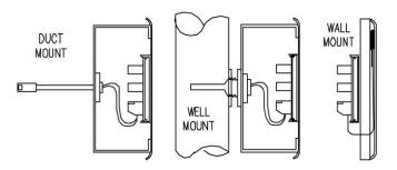
The AD590 sensor can be mounted in an 8'' duct probe, 3-8'' deep well, or in a Vandal Resistant Wall Mount (VRWM) sensor housing. The UMATR 2 wire transmitter is used when distances exceed 100+ feet exist between sensor and controller.
