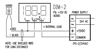
The AD590 sensor can be used in a standalone temperature INDICATION BY USING A +15VDC SUPPLY AND A DIM3 LCD display.
