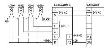
The SIA07 can be configured for up to five AD590 sensors and then select either the highest or lowest temperature, or average temperature. The SIA07 provides the + 15VDC reference voltage and load resistors for each sensor.
