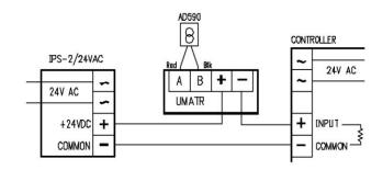
The AD590 sensor with a UMATR 4-20mA 2 wire loop transmitter, is used for long signal runs and in electrically noisy environments.
