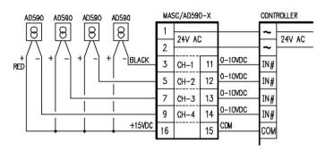
The MASC 4 channel signal converter permits the AD590 sensors to be used with any DDC Controller. Each channel can be customized for a variety of temperature ranges. The MASC provides the + 15VDC reference voltage and load resistors.
