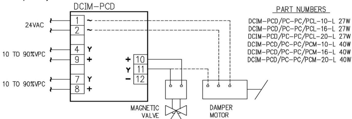
APPLICATION 8 - TWO MA SIGNALS LOW / HIGH SELECT TO PHASE CUT OUTPUT
