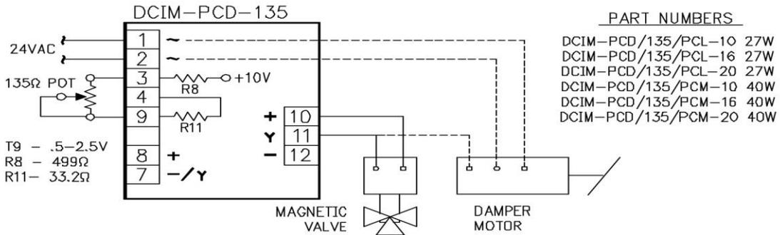
**APPLICATION 6 - VOLTAGE / CURRENT TO PHASE CUT CONVERSION**
