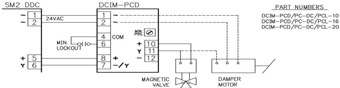
APPLICATION 4 - PHASE CUT WITH EXTERNAL MINIMUM POSITION POTENTIOMETER
