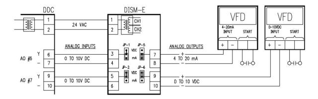
The DISM-E/2/SEL can convert two 0-10VDC or 4-20mA signals to two 4-20mA or 0-10VDC output signals. The output signals are isolated from each other and from the two input signals. These isolated signals can be used to drive Variable Frequency Drives, valve or damper actuators. The on-board isolation transformer provides three independent power supplies to power the input section and both output sections avoiding any ground loop potentials.
