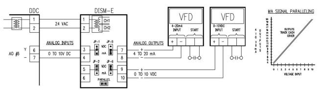
The DISM-E/2/SEL can be field configured by jumpering the parallel jumper for parallel output operation (standard), for parallel operation, connect control signal to channel 1 (IN1+/-), select input type Jp1, select parallel jumper, select output action (Jp3,4 D/R) for each output, and output signal type (VDC or mA) for each output. The on-board isolation transformer provides isolation between the two VFDs and the voltage or current output of the DDC controller.
