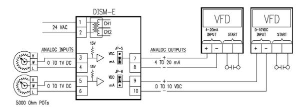
The DISM-E/PK5 is factory configured for two 5000 Ohm potentiometer inputs to provide a 0-100% control of two 4-20mA or 0-10VDC output signals. The output signals are isolated from each other and from the two input signals. These isolated signals can be used to drive Variable Frequency Drives, valve or damper actuators. The on-board isolation transformer provides three independent power supplies to power the input section and both output sections avoiding any ground loop potentials.
