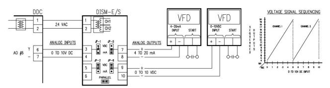
The DISM-E/2/SEQ is factory configured for sequencing operation. For sequencing operation, connect control signal to channel 1 (IN1+/-), select input type Jp1, verify parallel jumper in made, select output action (Jp3,4 D/R) for each output, and output signal type (VDC or mA) for each output. The on-board isolation transformer provides isolation between the two VFDs and the voltage or current output of the DDC controller.
