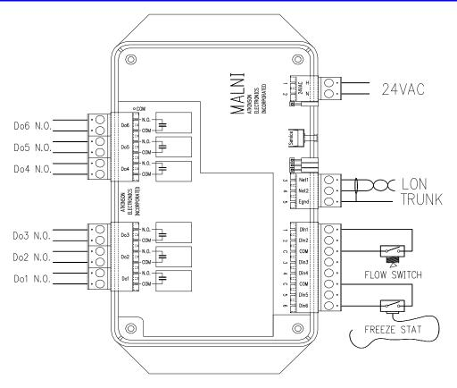
The above application wiring diagram for the MALNI-DO shows typical wiring for various digital outputs located below the 10 analog input terminals. Each of the outputs are normally open 1 Amp relay contact. If a higher current rated contact is needed, it is recommended that a 10 Amp pilot relay be used to switch the higher load currents. The status of each digital output is reported back on the LON network.
